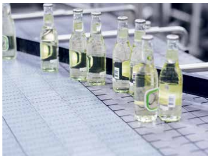
Bottles conveyor with FTDP1000 XLG MatTop® chain
