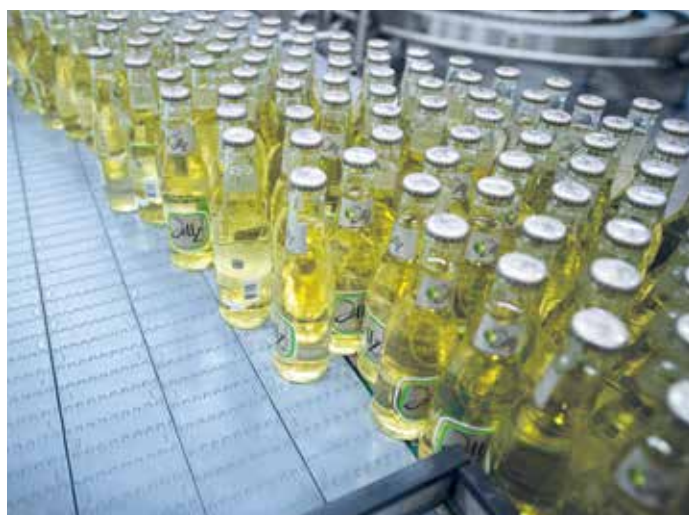
Bottles conveyor with FT1000 XLG MatTop® chain
